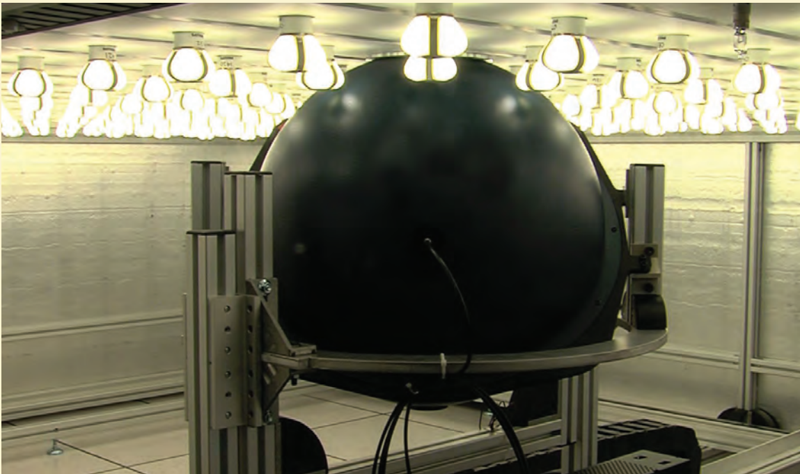
Long-term testing of the L Prize entry is being conducted in a specially designed high-temperature test bed.
